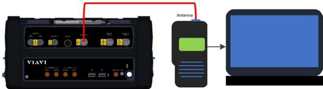
Figure 3-2 DMR Receiver Sensitivity Test Setup Diagram
