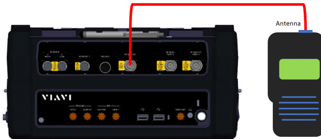
Figure 3-1 DMR Transceiver Test Setup Diagram
